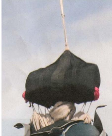
This is a line dump in process. Note the stretch of the rubber bands and that the canopy has already escaped the locking stows. Note also how the canopy is “slumped” in the bag. All of this is caused by inertia. This is a tandem with a collapsed drogue and large rubber bands which should produce a reduced Snatch. How much force do you think it takes to stretch those rubber bands?
